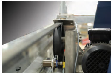
Rollers Inside Bridge and trolley movements are smooth and effortless using internally mounted dual-axis rollers. The hanging design enhances self-centering and improved roller life by protecting the rollers from the harsh wash environment.
