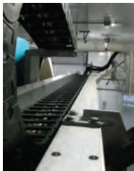
E-Chain Left or right mounted energy chain for easy and low-cost installation
