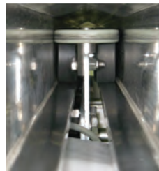
Rollers Inside Bridge and trolley movements are smooth and effortless using internally mounted dual-axis rollers. The hanging design enhances self-centering and improved roller life by protecting the rollers from the harsh wash environment.
